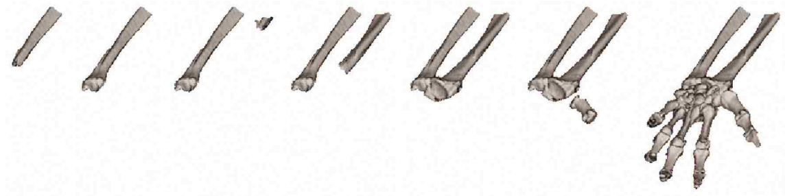
Figure 3.16: Evolving, growing surface. Selecting the bones in the arm and hand by dragging the mouse over them in the voxel display. The result is an evolving surface that appears to be growing.
